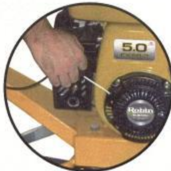
Self-rewinding recoil start
